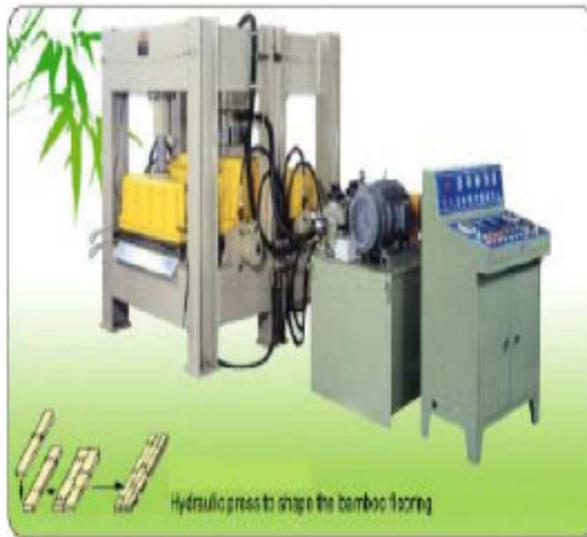
Name: BAMBOO FLOORING/BOARD JOINING MACHINE
