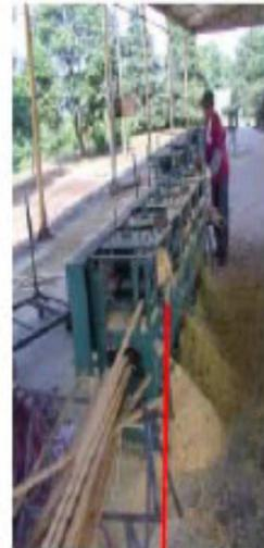
Name: BAMBOO STRIP 2-SIDES REMOVING MACHINE
