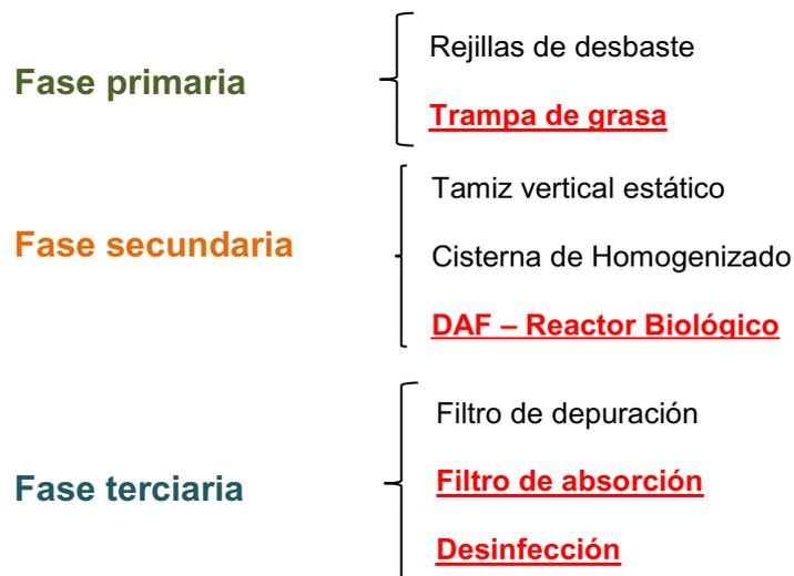
**Figura 4.1** Diseño conceptual de la restructuración
