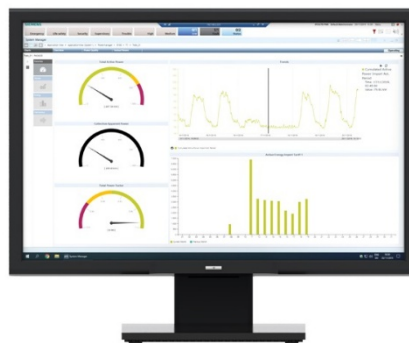
Figura 9 Software PowerManager de Siemens.
